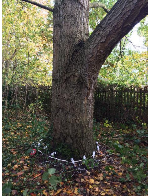
Photo 6: Showing sensors attached to stem base of T192
