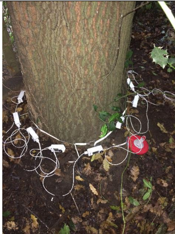
Photo 5: Showing sensors attached to stem base of T185
