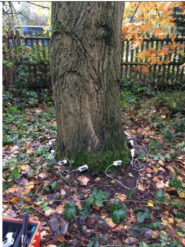
Photo 7: Showing sensors attached to stem base of T197
