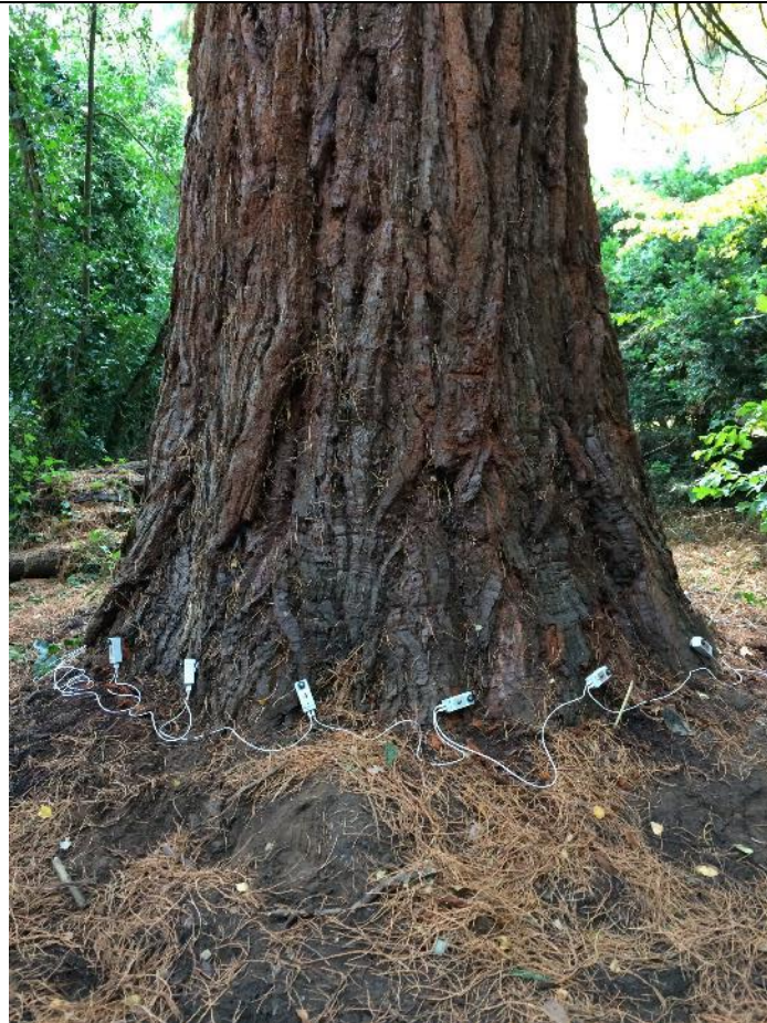
Photo 3: Showing sensors attached to stem base of T183
