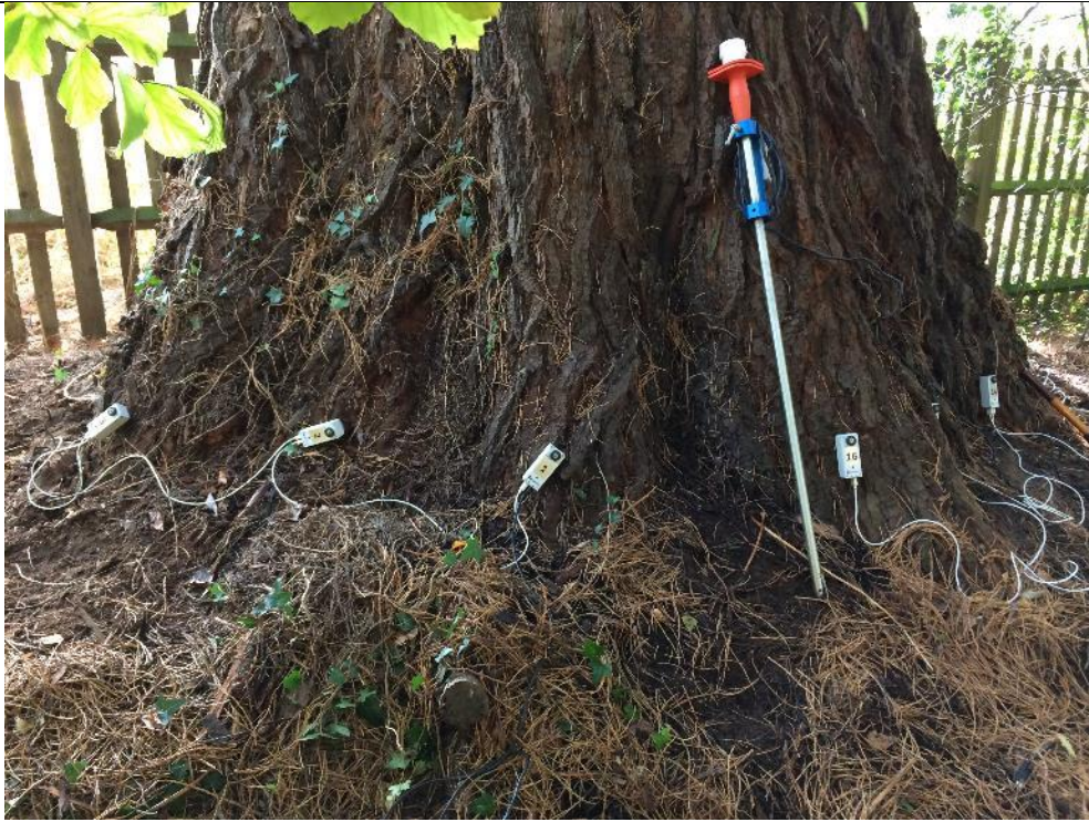
Photo 4: Showing sensors attached to stem base of T184
