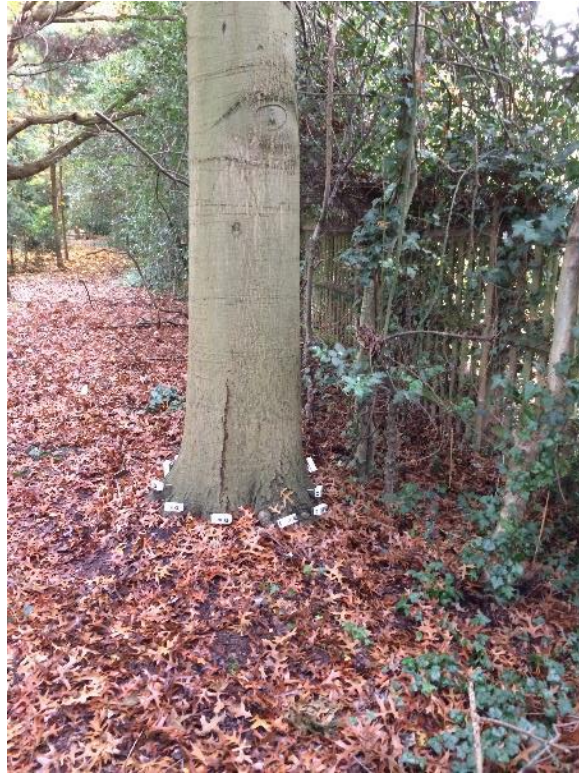
Photo 2: Showing sensors attached to stem base of T181
